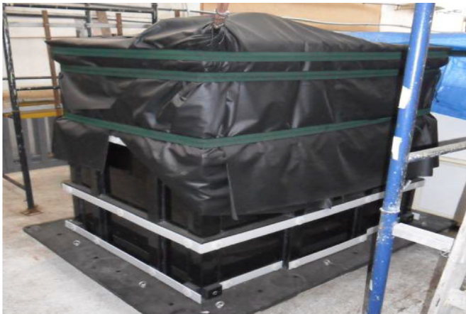
Fig. 8. Picture of the assembled detector, filled with water and sealed.
