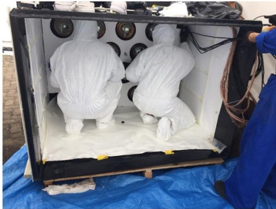
Figure 6. Bottom of the Target detector being instrumented in the nuclear power plant.
