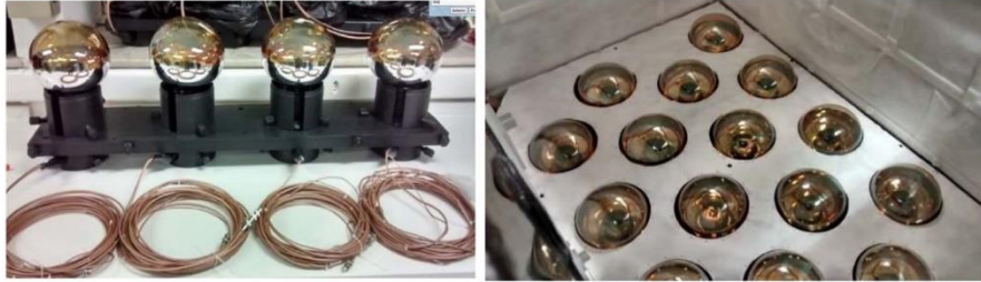
Fig. 7. Four PMTs on the mechanical support just before their installation inside the target detector (left) and the 16 PMTs installed on the bottom part of the target detector (right).
