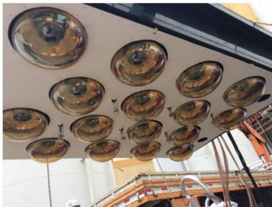
Figure 7. Target detector lid with the 16 PMTs and 6 LEDs installed.
