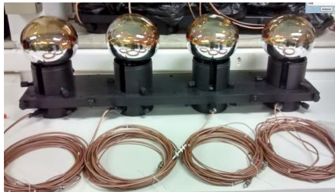
Figure 1: Four PMTs on their support before installing them inside the target detector.
