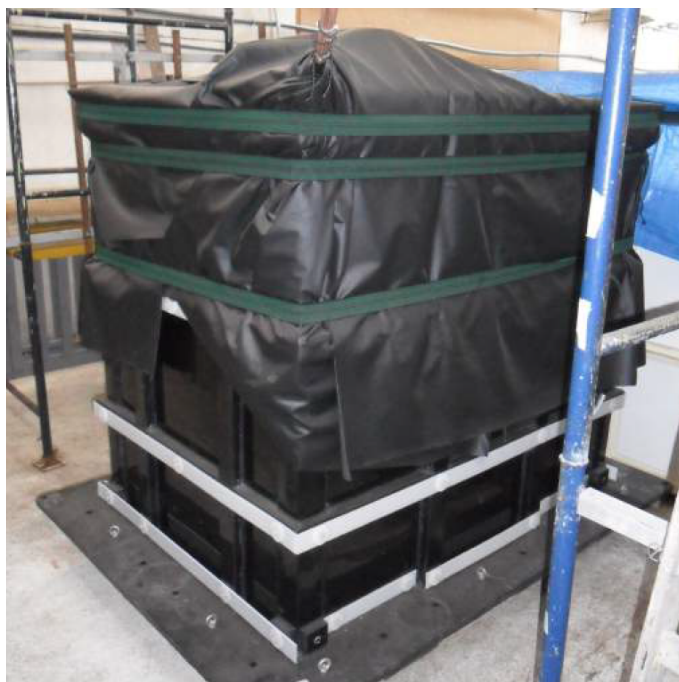
Figure 3: Picture of the detector assembled, filled with water and sealed.
