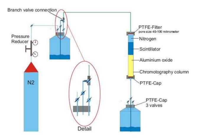
Figure 2: Oxygen free column chromatography purification setup.
