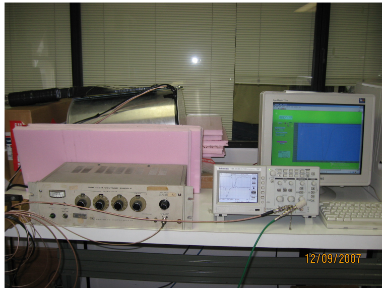
Figure 2: Photograph of the experimental setup showing the dark chamber in a horizontal position with the scintillation paddle on top of it (upper left corner), the HV power supply, the digital oscilloscope (Tektronix TDS1012B) and the PC monitor.
