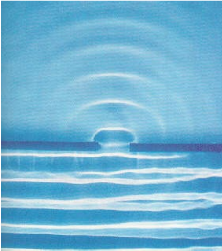
Water waves in a tank with a single slit aperture.
