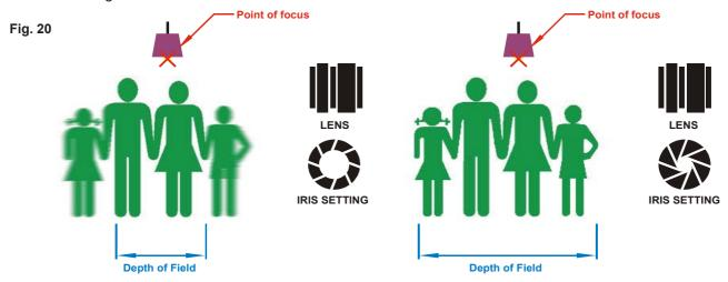
One disadvantage of increasing the depth of field by closing the iris, is the amount of light admitted to the camera will be reduced and the image will become darker. Depth of field is also dependent upon the focal length of the lens. Wide angle lenses (i.e. those with a small focal length) will have a greater depth of field than telephoto types. The depth of field is inversely proportional to the focal length of the lens so as focal length increases, the depth of field will decrease.
