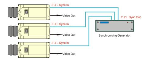
Baxall cameras also have an internal oscillator which is selected using the **Internal** mode switch. This feature can be especially useful where the camera is designed to run off a D.C. supply or if a camera designed to operate at 50Hz (e.g. PAL standard), is installed in a country where the mains supply frequency is at 60Hz. Ordinarily the camera would not be able to use the Line Lock mode. Setting it to synchronise to its internal oscillator will overcome this
