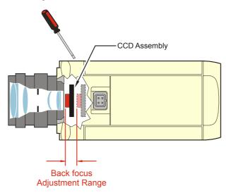
NOTE: It is important that the lens iris is fully open before the back focus is set. This is because the depth of field will be at its minimum and won't be tending to 'focus' the image.
